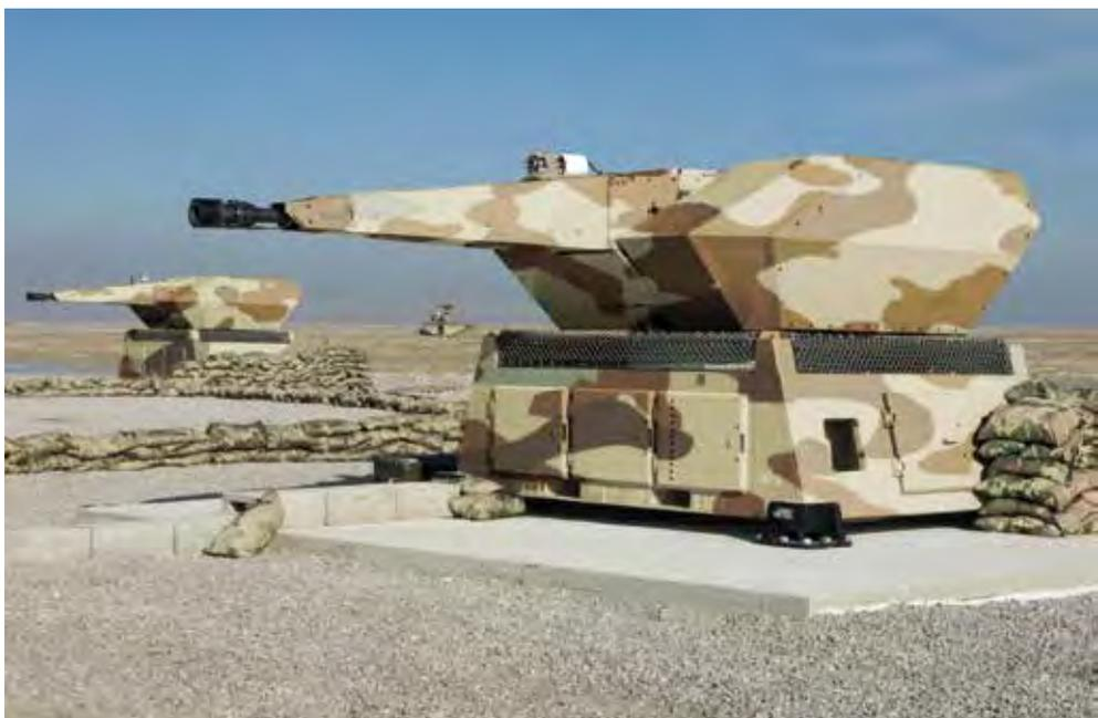
**The Rheinmetall Air Defence Oerlikon SKYSHIELD air defence system is mounted on pallets so it can be rapidly deployed where it is required. The picture shows the two revolver gun mounts with the sensor unit with surveillance and tracking radars to the rear.**
