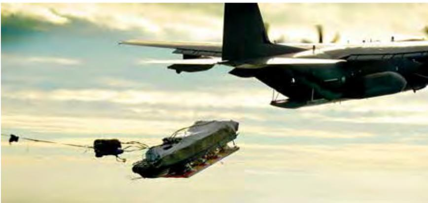
**The Maritime Craft Aerial Delivery System (MCADS) deploys via the ramp to fly to its target destination. Immediately after, the boat crew and US Navy SEALs will follow.**
