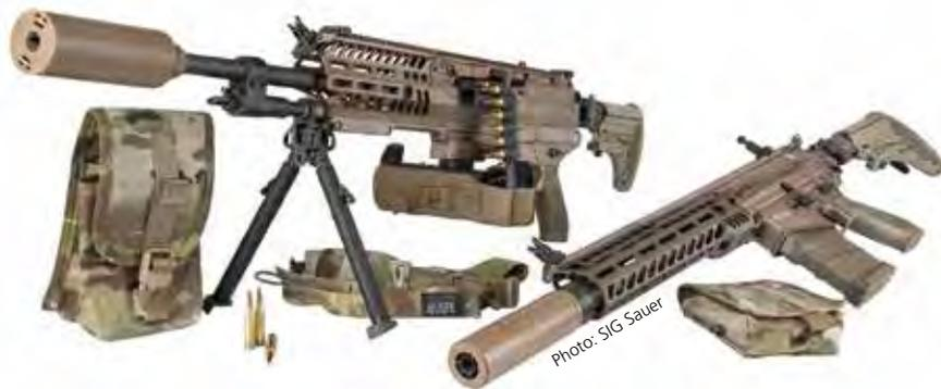
**SIG Sauer developed a new lightweight machine gun and carbine, chambered in 6.8 mm hybrid ammunition for increased penetration at greater distances with increased velocity and accuracy.**
