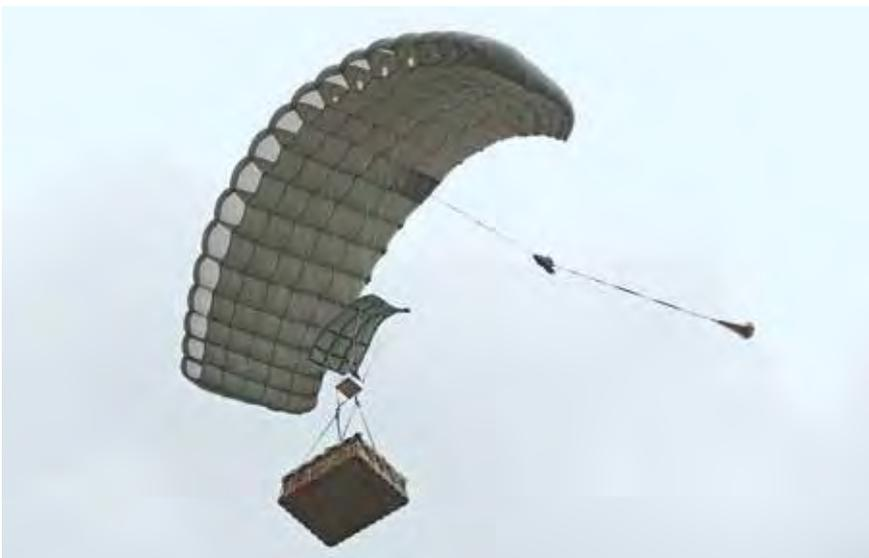
**The Airbus PARALANDER is a fully autonomous GPS guided cargo delivery system. It can carry up to 1,000 kg.**
