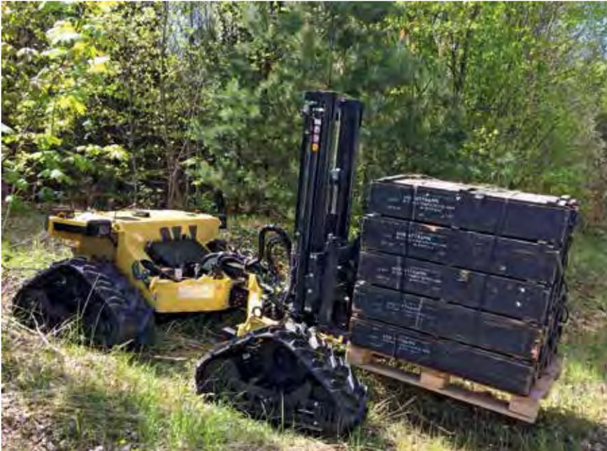
**The Palfinger CRAYLER can move material up to 1,400 kg in all kinds of conditions.**
