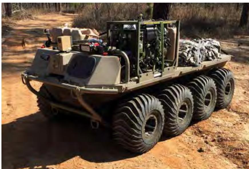
**The Lithium Battery Company (LBC), which supplies batteries for GDLS’ MUTT unmanned ground vehicle (UGV) for the US Army’s Small Multi-Purpose Equipment Transport (SMET) requirement, invented an exclusive BMS that is programmable to meet the high endurance battlefield requirements for the MUTT UGV. The proprietary BMS technology can be monitored in real-time through an on-board computer, creating the ability to adjust performance parameters from anywhere in the world.**
