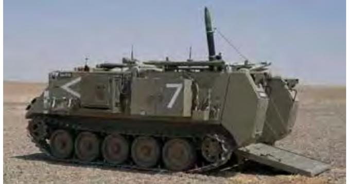
**The IRON STING that has recently completed trials with the Israel Defense Force (IDF) is a 'networked precision fire system' enabling the infantry battalion firing mortar munitions with high precision, using a combination of laser and GPS guidance.**
