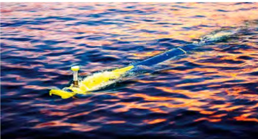
**The Saab AUV62 MR is the mine reconnaissance variant of the 53.3 cm diameter AUV62 family of UAVs, which also includes target and mine variants.**
