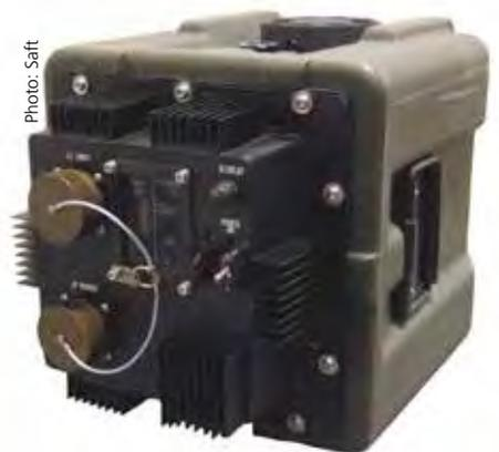
**Based on the 28V Lithium Battery Box (LBB) developed for the US Army's TOW Missile, the high-power LBB is a 28 V, 100 amp-hour battery made up of high-energy Li-ion cells.**
