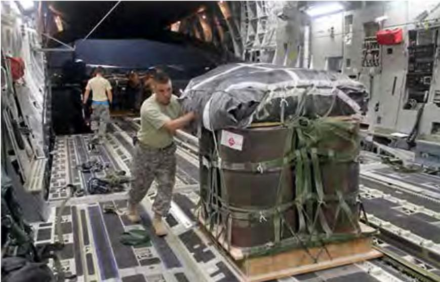
**Parachute riggers load pallets into a C-17 aircraft. Container delivery systems help to make this process easier and faster.**
