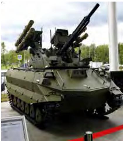
URAN-9 is also armed with a 30-mm automatic cannon and six ready-to-launch SHMEL reactive flame launchers. There are two ATAKA missile launchers and three SHMEL launchers on each side of the turret. URAN-9 is powered by a diesel-electric engine providing maximum speed of 35 km/h on roads, slowed down to 10 km/h in off-road conditions.
